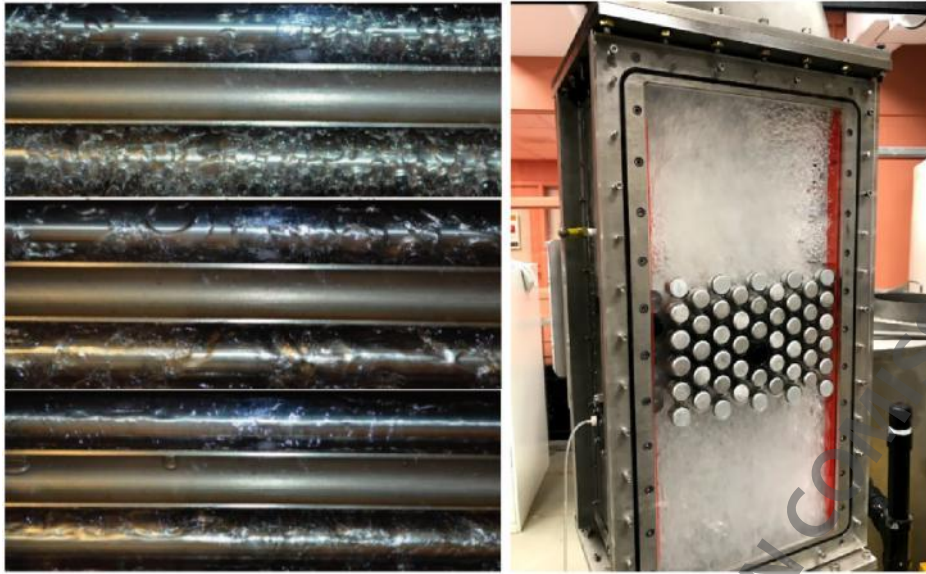
Figure 24: Side view of a dispersed flow in a triangular tube bundle from Kanizawa et al. (2016) [106] and view of the test section from Darwish et al. (2023) [107] for a high void fraction.
